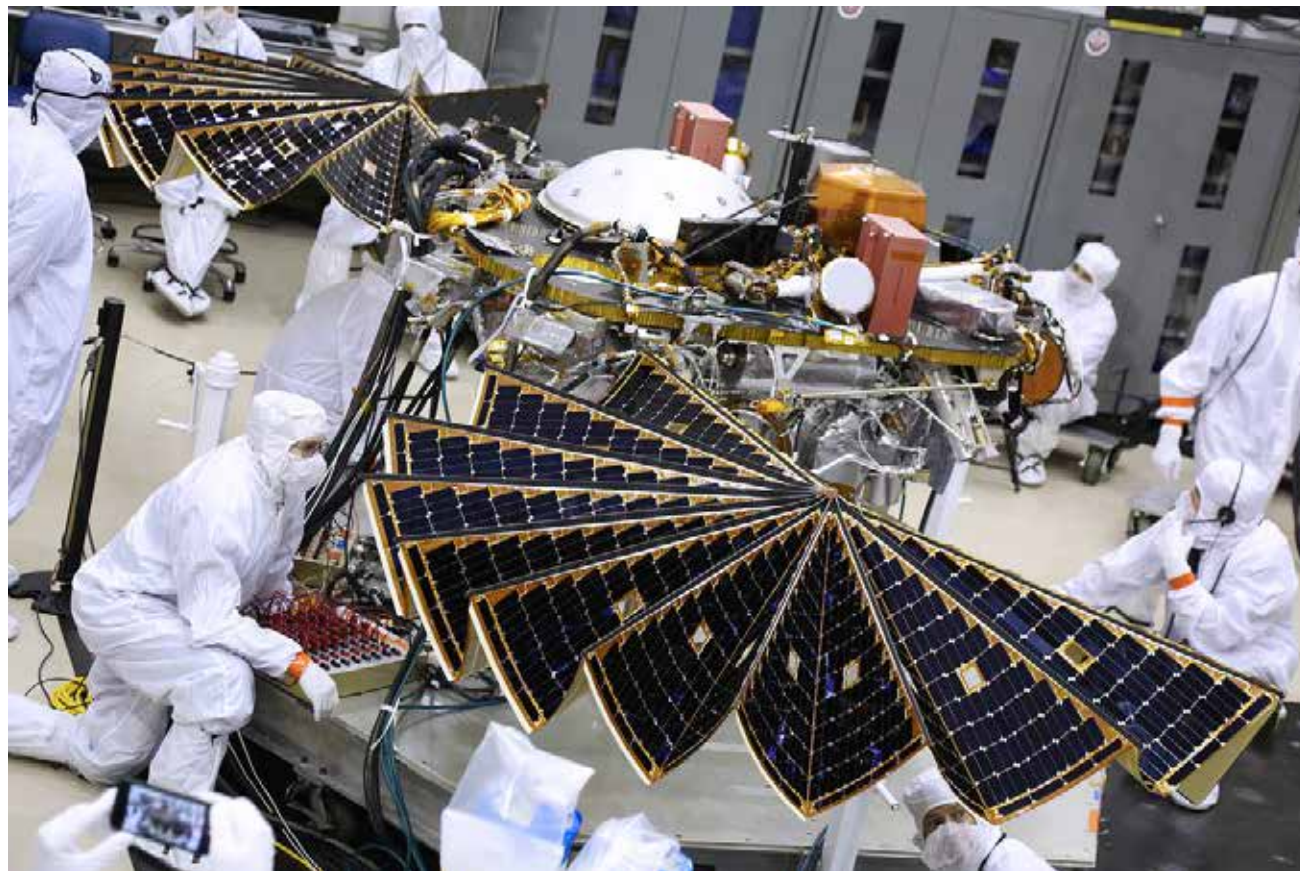
Testing the InSight Mars Lander's solar arrays Image credit: Lockheed Martin Space
