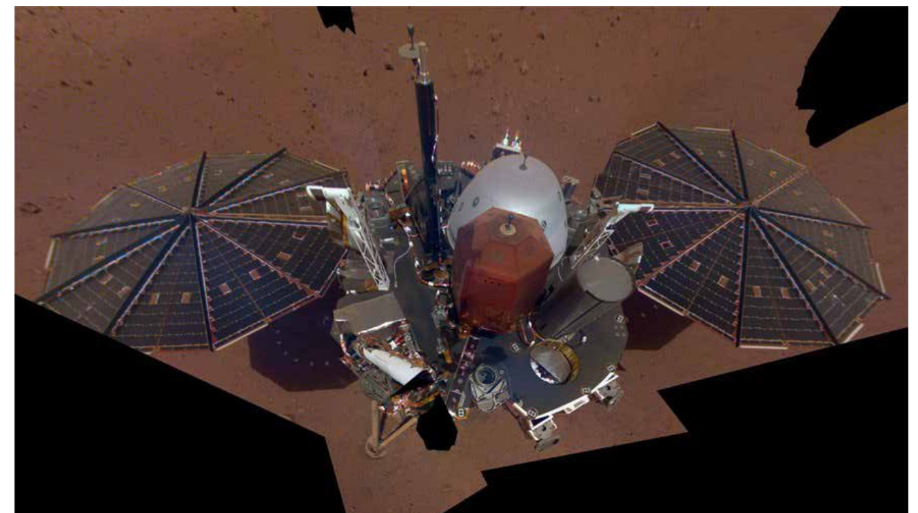
This is NASA InSight's first full self-portrait on Mars. It displays the lander's solar panels and deck. On top of the deck are its science instruments, weather sensor booms and UHF antenna. The selfie was taken on Dec. 6, 2018. Image credit: NASA/JPL-Caltech.
